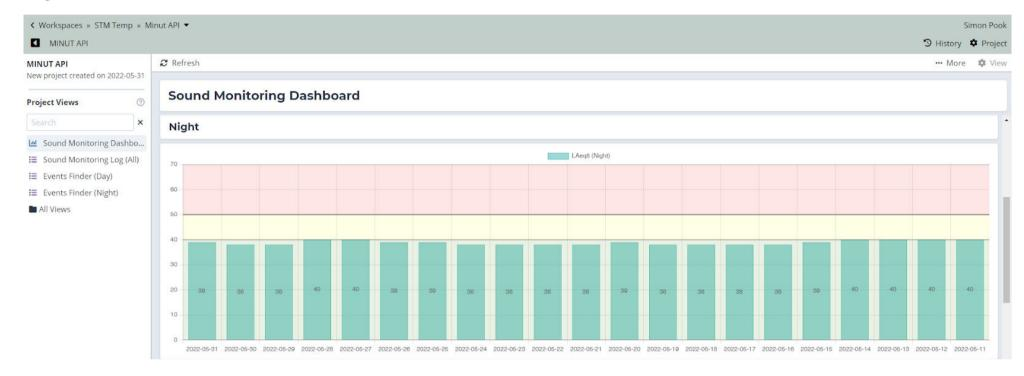
Noise floor of 36dB has an impact with these results since the unit is unable to measure below that value.
