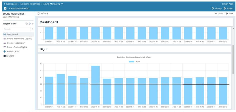
Noise floor of 36dB has an impact with these results since the unit is unable to measure below that value. The requirement of 30dB Laeq, 8 (8 is the number of continuous hours)
